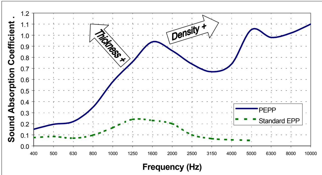
Note: Test Samples: Density = 2.8 pcf (45 g/l) and Thickness = 30 mm (1.2").
