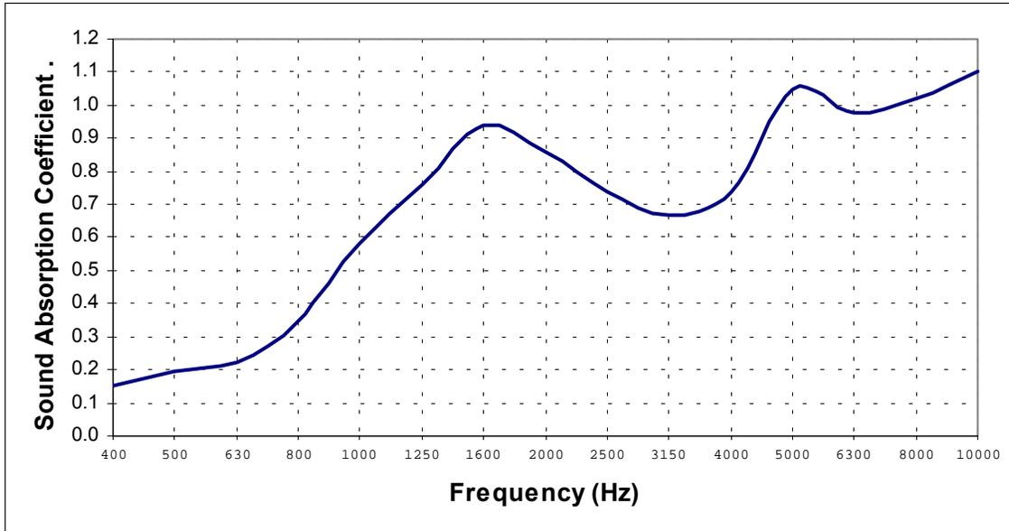
Note: Test Sample Thickness = 30 mm (1.2")
